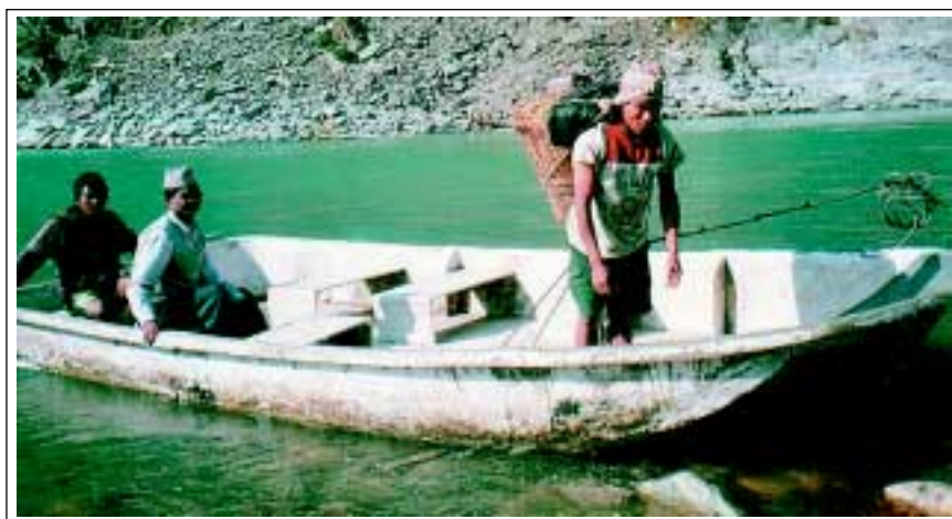
■ Natural-force ferry boat in operation in Ghatbesi, Trisuli.
